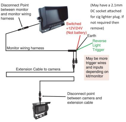
The above diagram shows the basics of how your kit will be laid out. If you have ordered a trailer link or more than one camera then the setup will be slightly different. If using the trigger wire and it only has one then ensure the camera cable is in Channel 2. If your monitor has more than one trigger wire then they should be labelled channel 1/2/3 etc so you can choose which trigger you wish to put to which camera channel.
